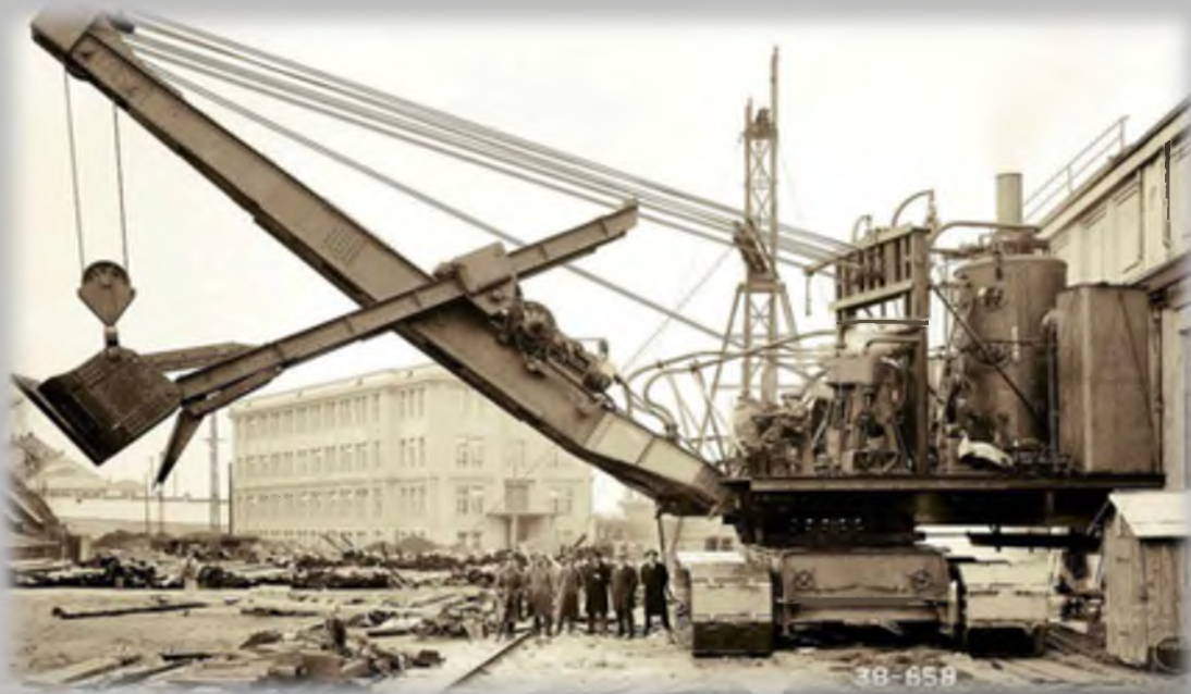
1926 Pasove Rypadlo huge steam shovel at 220 ton it dwarfs the guys below
