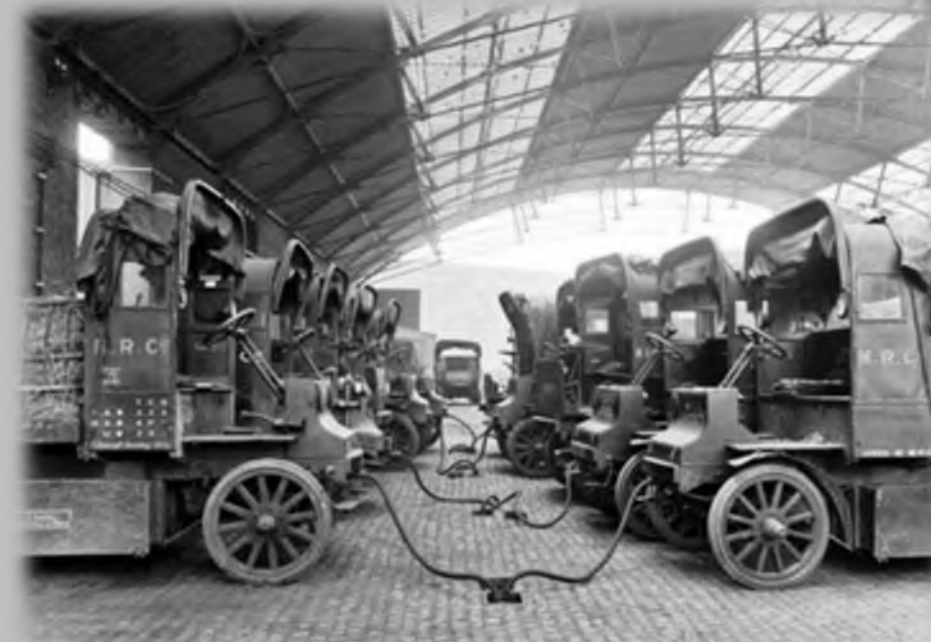
1917, electric at charging terminal in St Pancras, London. Who said electric vehicles are a new phenomenon?
