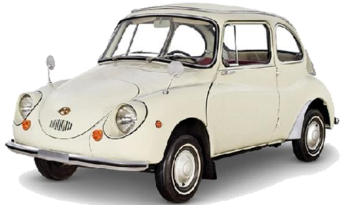
1958 Subaru 360. Twin-cylinder (two-stroke) 356cc 16hp
