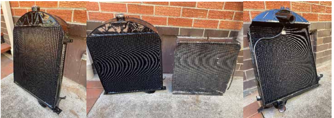
Comparison of the Original Core and Re-Cored Radiator, chalk & cheese
