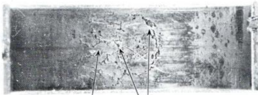
Fig. 2.9.14—Effect of large hard particle which has travelled around the bearing several times.
