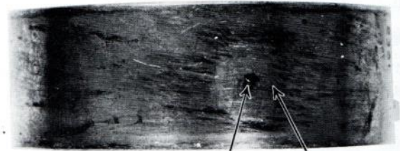
Fig. 2.9.14—Effect of large hard particle which has travelled around the bearing several times.
