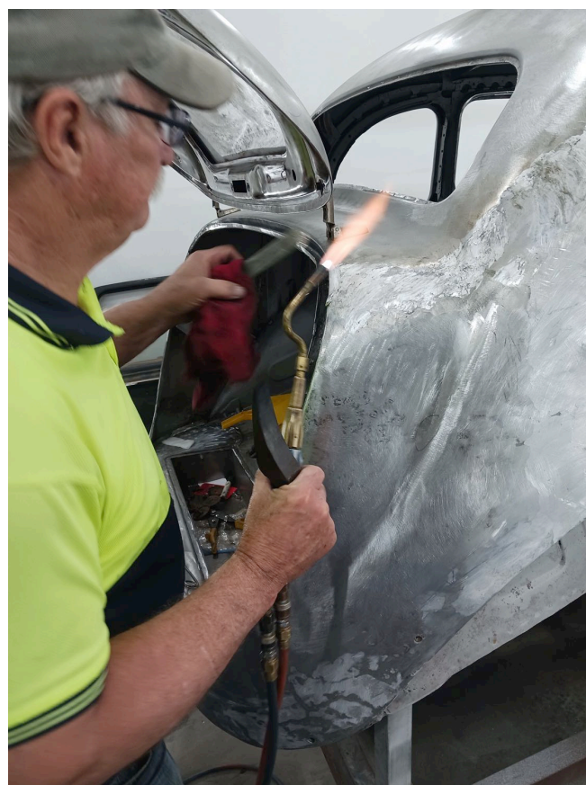
Les repairing the original lead wiped sections.
