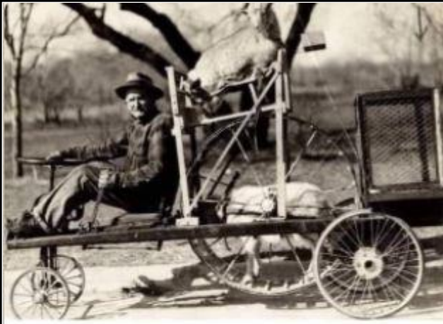
An American farmer demonstrates his goatmobile. The vehicle is driven by a goat, which is in a running wheel. The goatmobile could reach speeds of up to 15 km/h. The spare goat at the top, 1937.
