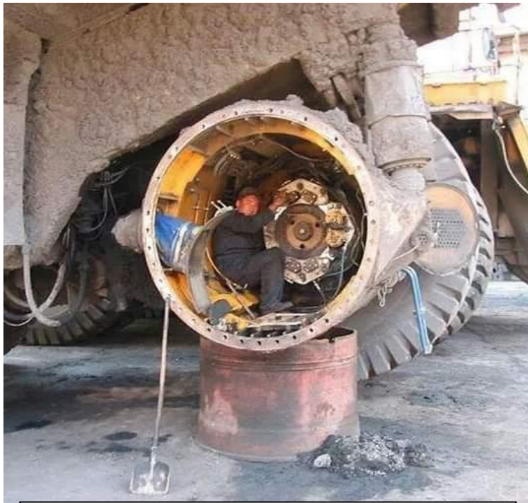
Working on a diff from a mining dump truck
