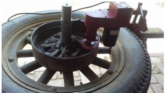
Grinding the brake drum concentric with home made jig supporting tool post grinder.
