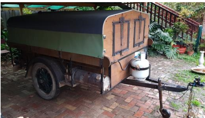
Near hatch opens onto three-way car fridge. Far hatch opens onto storage. Copper water tank, Dead easy tire pump and folding gas grill (at rear) are visible on this side.
