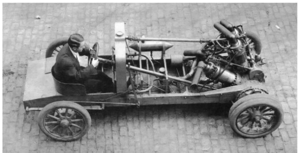
From above the unusual layout of the V4 is even more evident. There appears to be no gearbox! The car must have had so much torque that it didn't need one. The photos taken in the shop suggest gear change mechanisms at the very front of the engine.
