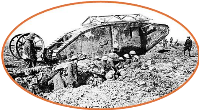
Mark I tank during the Battle of the Somme Daimler-Knight 6-cyl 105hp sleeve-valve 16-litre petrol engine
