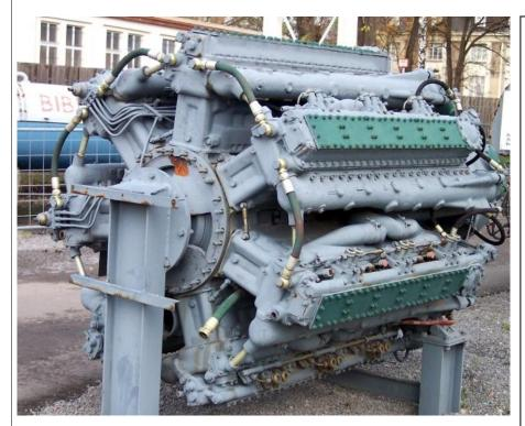
The Yakovlev M-501 was a large, water-cooled, diesel, four-stroke, aircraft engine. The 42-cylinder engine was an inline radial configuration consisting of seven cylinder banks positioned around an aluminium crankcase. The crankcase was made up of seven sections bolted together: a front section, five intermediate sections, and a rear accessory section. The crankshaft had six throws and was supported in the crankcase by seven main bearings of the roller type.
