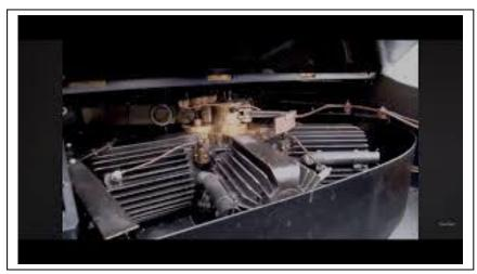
This Engine rotated around the crankshaft, this meant the cylinders rotated so there was no need for a flywheel. The Adams-Farwell Company of Dubuque, lowa produced automobiles from 1905 through 1913. Herbert and Eugene Adams founded the company in 1883 for the purpose of producing park benches and grave markets. Their business evolved over the years to include milling and general foundry equipment.
